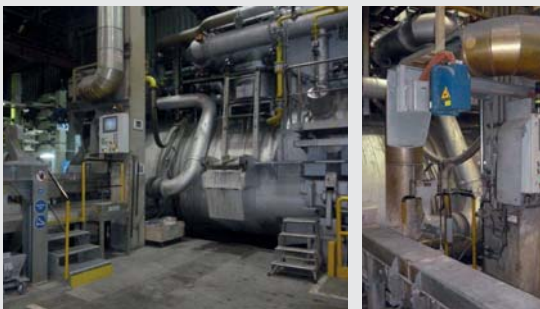
Left: Light-metal foundry at BMW's Landshut factory Right: TPCC®-protected sensor monitoring the fill-level
